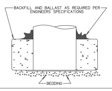
TANK VOLUME (INTERNAL) = 15.7 cu ft/117.5 gal TANK WEIGHT W/LID = 71 lbs
