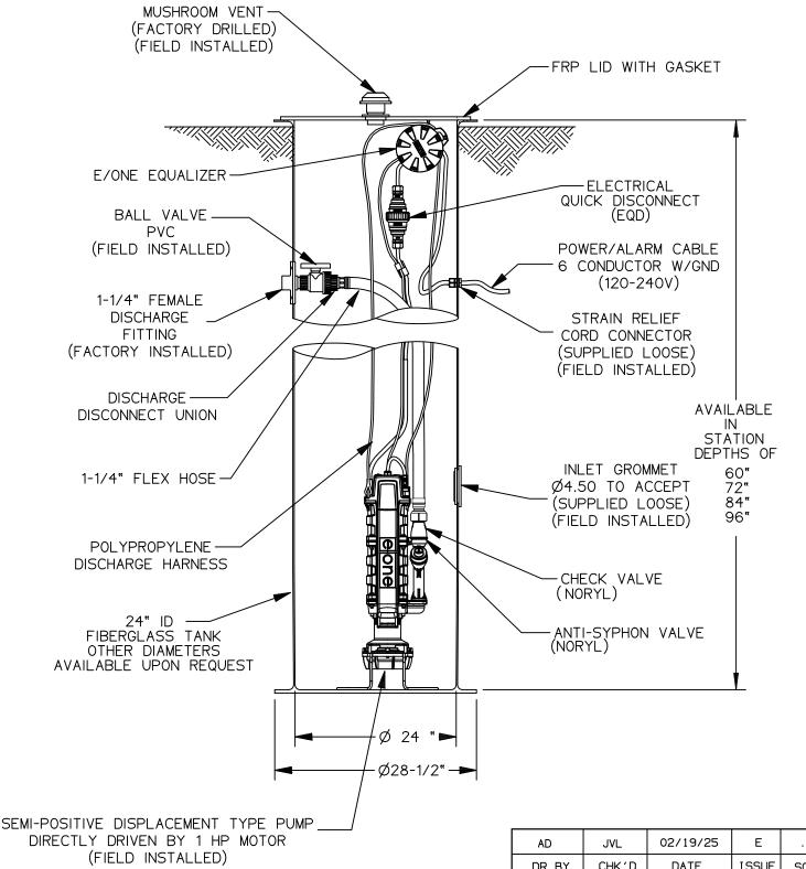
NOTE: BALLASTING IS REQUIRED TO PREVENT TANK FROM FLOATING. INSTALL CONCRETE ANCHOR PER ENGINEERS RECOMMENDATIONS
