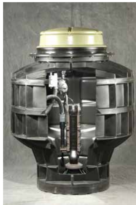
Featuring the E/One Extreme grinder pump, the WH231/WR231 offers a high level of reliability and ruggedness. The lower portion of the tank has a smaller diameter, tapered down to a dish-shaped bottom. These design features reduce the retained volume and promote scouring, which will minimize odor and corrosiveness.
